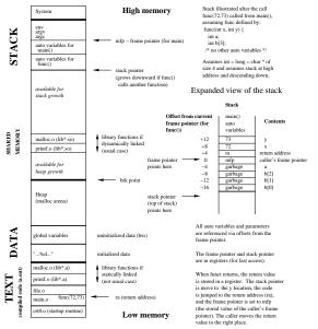
Memory Layout (Virtual address space of a C process)
